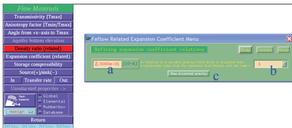
Figure 1.5 Input of the so-called related density parameters: a) solute density ratio or expansion coefficient constant(s), b) a link to the reference distribution containing the z -coordinates of the aquifer, and c) preview of the resulting projected gravity field.
